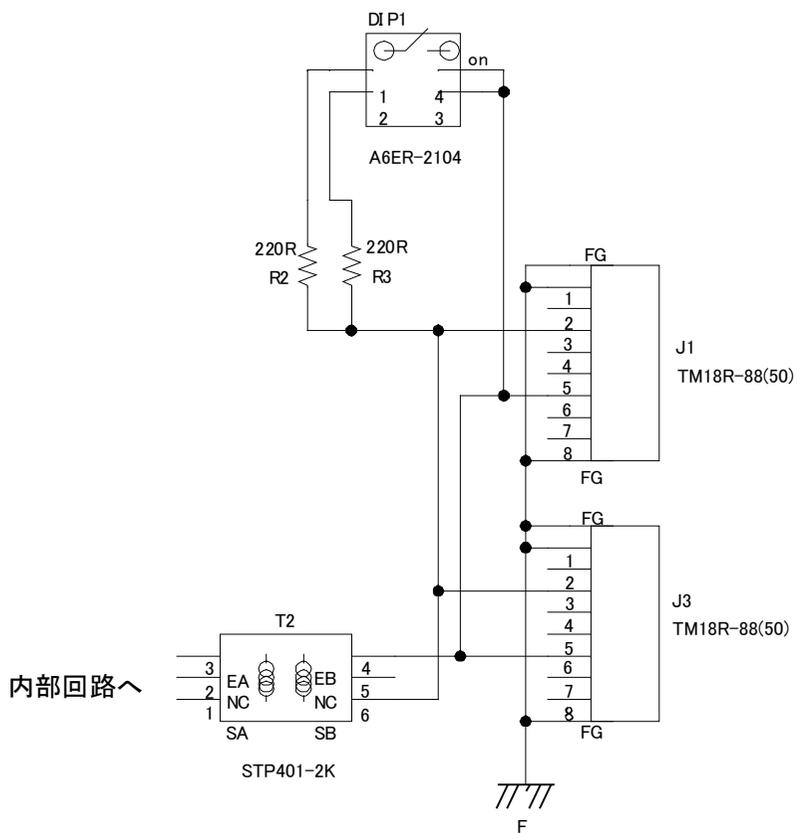
\*Communication line is isolated from the internal circuit with a pulse transformer (T2).
