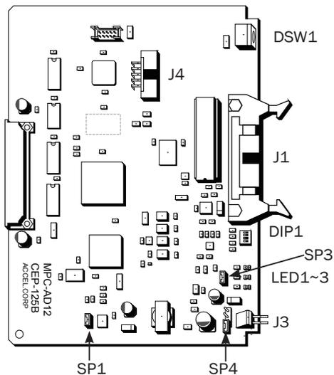
\* SP1 is for the internal AD/DA power supply (OFF if unnecessary).
