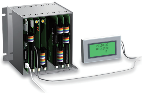
The 8 slots system case CH1: connected to the MPC-IP CH2: connected to a touch panel display
