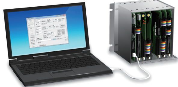
A MPC system with a PC A PC and a MPC-IP can be connected by setting fix IP address for both of them.
