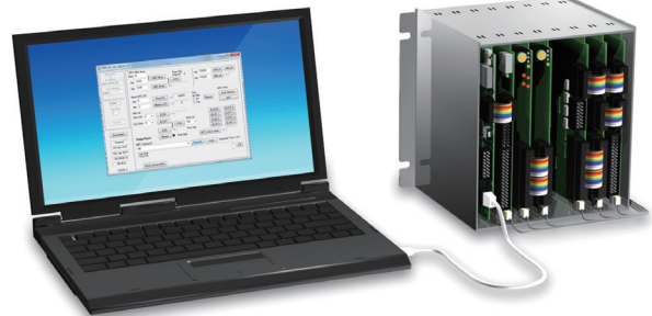
A MPC system with a PC A PC and a MPC-IP can be connected by setting fix IP address for both of them.
